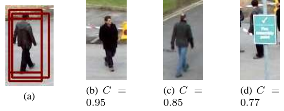
Figure 4: Confidence computation : (a) set of candidates for one person; (b) : a perfectly detected individual with a high confidence; (c) : an uncertain detection with an average confidence ; (d) : a bad detection with a low confidence due to occlusion.
