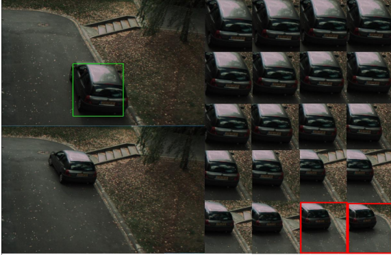
Figure 3. Car tracking results (every 5th frame) using: the covariance descriptor (upper image) and the Brownian descriptor (bottom image).
